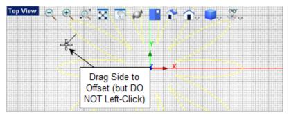
Now with the curve offset direction displayed enter 0.5 in the command input bar Command sand press the <Enter> key. The curve will be offset toward the outside by 0.5 inches.
