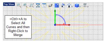
15. Now from the Curve Modeling command. This will merge all of the curves into one curve. This makes it easier to work with. Only curves that are joined end to end will be merged. Separate curves such as those created from the section of the outer spheres will remain separate curves.
