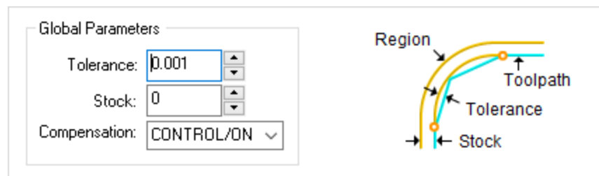
Tolerance value on the Cut Parameters tab for 2 ½ Axis Profiling
