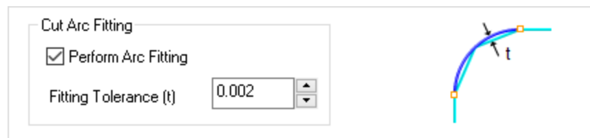
Perform Arc Fitting on the Advanced Cut Parameters tab for 2 ½ Axis Profiling
