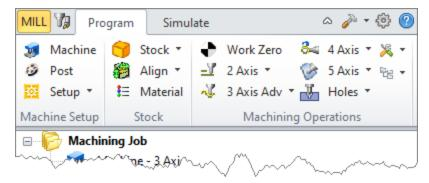
2. From the Machining Job tree select the operations that your wish to post a G-Code file for. If you have an automatic tool changer on your CNC machine you can post all operations in one file by selecting Setup 1.
