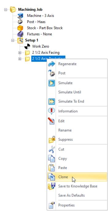
3. This will create a copy of the operation and place it below the original in the Machining Job. Now right-click on the second operation and pick Edit.
