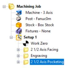
12.In 2½ Axis Pocketing an additional display toggle icon appears on the Machining Job toolbar (at the bottom). Select it to open the Z Level Display dialog that allows you to select and view each cut level in the Pocketing operation as shown below.
