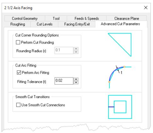
11. Now pick Generate and the 2½ Axis Facing toolpath is calculated and displayed on the part. It is also listed in the Machining Job under the Work Zero. The part and Machining Job are shown below.
